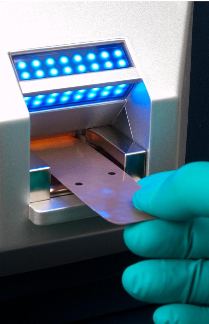
The new Bruker DE-tector is the latest innovation in trace narcotics and explosives detection. It is the first table top device with a combined non-radioactive ionisation source and a unique third generation twin tube IMS design.
