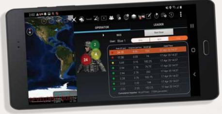
**Mobile Connectivity:** The Blast Gauge System App (BGSA) for Android™ allows for near real-time data analysis and download with Bluetooth 4.1
